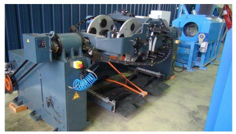
Equipment designed to produce high quality communication pairs (LAN or other) based on group twinner technology ie two pay-off bobbins are mounted inside rotating bow. By just adding a take-up, a complete twinning line will be designed.
